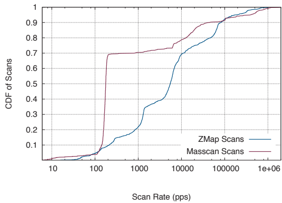
Figure 6: CDF of scan rate — The fastest scans operated at 2.2 Mpps (about 1.5 Gbps). However, less than 10% of scans exceeded 100 Mbps.
